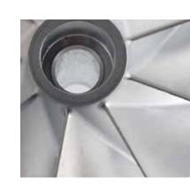
Quantima's<sup>™</sup> patented Q-drive<sup>™</sup> compression and motor assembly has just one moving part and operates with the rotor spinning in a magnetic field at up to 60,000 rpm.
